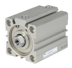
NITRA pneumatic cylinder, compact extruded, 40mm bore, 16mm rod diameter, 30mm stroke, double acting, magnetic piston, tapped end caps mount.
