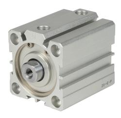
NITRA pneumatic cylinder, compact extruded, 40mm bore, 16mm rod diameter, 25mm stroke, double acting, magnetic piston, tapped end caps mount.
