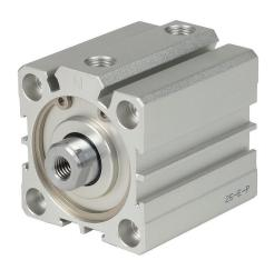
NITRA pneumatic cylinder, compact extruded, 40mm bore, 16mm rod diameter, 20mm stroke, double acting, magnetic piston, tapped end caps mount.
