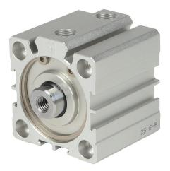
NITRA pneumatic cylinder, compact extruded, 40mm bore, 16mm rod diameter, 10mm stroke, double acting, magnetic piston, tapped end caps mount.
