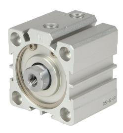
NITRA pneumatic cylinder, compact extruded, 40mm bore, 16mm rod diameter, 5mm stroke, double acting, magnetic piston, tapped end caps mount.
