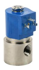
GC Valves solenoid valve, 2-port (2-way), 2-position, N.C., stainless steel body, Viton/PTFE seal(s), 3/8in female NPT inlet(s), 3/8in female NPT outlet(s), Cv=1.5, 0 psi minimum operating pressure, 24 VDC operating voltage, 18mm DIN style wiring plug.
