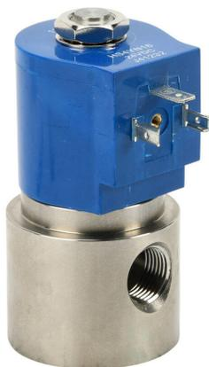
GC Valves solenoid valve, 2-port (2-way), 2-position, N.C., stainless steel body, Viton/PTFE seal(s), 3/8in female NPT inlet(s), 3/8in female NPT outlet(s), Cv=1.5, 0 psi minimum operating pressure, 24 VDC operating voltage, 18mm DIN style wiring plug.
