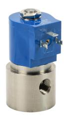
GC Valves solenoid valve, 2-port (2-way), 2-position, N.C., stainless steel body, Viton/PTFE seal(s), 1/4in female NPT inlet(s), 1/4in female NPT outlet(s), Cv=1.1, 0 psi minimum operating pressure, 24 VDC operating voltage, 18mm DIN style wiring plug.
