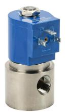
GC Valves solenoid valve, 2-port (2-way), 2-position, N.C., stainless steel body, Viton/PTFE seal(s), 3/8in female NPT inlet(s), 3/8in female NPT outlet(s), Cv=1.5, 0 psi minimum operating pressure, 120 VAC operating voltage, 18mm DIN style wiring plug.
