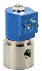
GC Valves solenoid valve, 2-port (2-way), 2-position, N.C., stainless steel body, Viton/PTFE seal(s), 1/4in female NPT inlet(s), 1/4in female NPT outlet(s), Cv=1.1, 0 psi minimum operating pressure, 120 VAC operating voltage, 18mm DIN style wiring plug.
