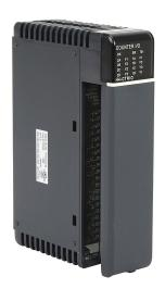
DirectLOGIC DL405 pulse combo module, 100 kHz maximum switching frequency, 8 high-speed input point(s), sinking/sourcing, single-ended encoder input(s), 4 high-speed output point(s), sinking/sourcing, single-ended output(s).
