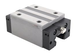
WON H35 series standard bearing block, full ball recirculating, rectangular, end seal and inside seal, carbon steel. For use with H35 series rails.
