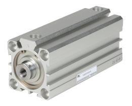
NITRA pneumatic cylinder, compact extruded, 32mm bore, 16mm rod diameter, 75mm stroke, double acting, magnetic piston, tapped end caps mount.
