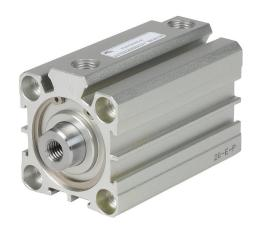
NITRA pneumatic cylinder, compact extruded, 32mm bore, 16mm rod diameter, 40mm stroke, double acting, magnetic piston, tapped end caps mount.
