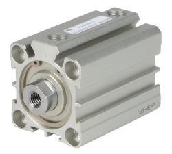
NITRA pneumatic cylinder, compact extruded, 32mm bore, 16mm rod diameter, 30mm stroke, double acting, magnetic piston, tapped end caps mount.
