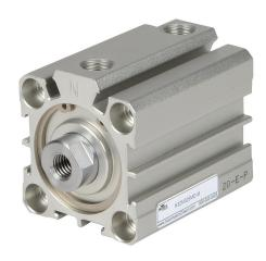
NITRA pneumatic cylinder, compact extruded, 32mm bore, 16mm rod diameter, 25mm stroke, double acting, magnetic piston, tapped end caps mount.
