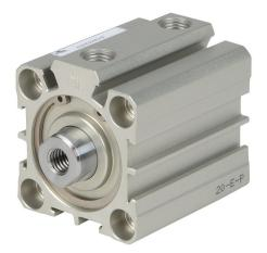
NITRA pneumatic cylinder, compact extruded, 32mm bore, 16mm rod diameter, 20mm stroke, double acting, magnetic piston, tapped end caps mount.
