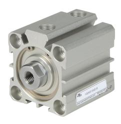
NITRA pneumatic cylinder, compact extruded, 32mm bore, 16mm rod diameter, 15mm stroke, double acting, magnetic piston, tapped end caps mount.
