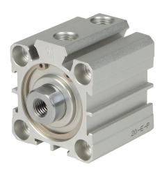
NITRA pneumatic cylinder, compact extruded, 32mm bore, 16mm rod diameter, 10mm stroke, double acting, magnetic piston, tapped end caps mount.
