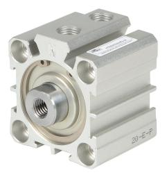
NITRA pneumatic cylinder, compact extruded, 32mm bore, 16mm rod diameter, 5mm stroke, double acting, magnetic piston, tapped end caps mount.
