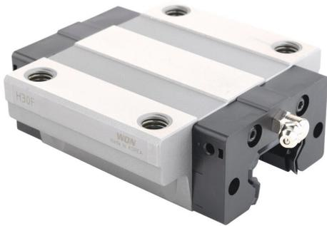
WON H30 series standard bearing block, full ball recirculating bearing, flanged, end seal and inside seal, carbon steel. For use with H30 series rails.
