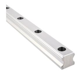
WON H30 series standard rail, carbon steel, 26 x 28 x 1000mm. For use with H30 series bearings.
