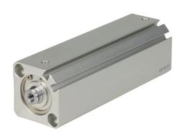
NITRA pneumatic cylinder, compact extruded, 25mm bore, 12mm rod diameter, 100mm stroke, double acting, magnetic piston, tapped end caps mount.
