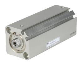
NITRA pneumatic cylinder, compact extruded, 25mm bore, 12mm rod diameter, 75mm stroke, double acting, magnetic piston, tapped end caps mount.
