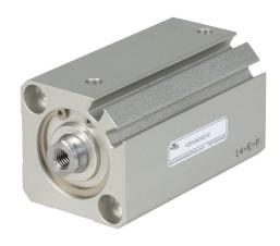
NITRA pneumatic cylinder, compact extruded, 25mm bore, 12mm rod diameter, 40mm stroke, double acting, magnetic piston, tapped end caps mount.
