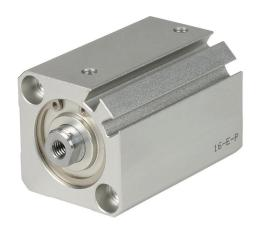
NITRA pneumatic cylinder, compact extruded, 25mm bore, 12mm rod diameter, 30mm stroke, double acting, magnetic piston, tapped end caps mount.
