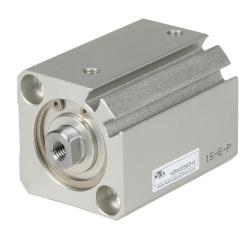
NITRA pneumatic cylinder, compact extruded, 25mm bore, 12mm rod diameter, 25mm stroke, double acting, magnetic piston, tapped end caps mount.
