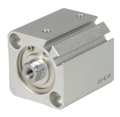
NITRA pneumatic cylinder, compact extruded, 25mm bore, 12mm rod diameter, 15mm stroke, double acting, magnetic piston, tapped end caps mount.
