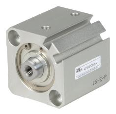
NITRA pneumatic cylinder, compact extruded, 25mm bore, 12mm rod diameter, 10mm stroke, double acting, magnetic piston, tapped end caps mount.
