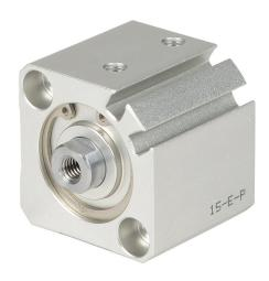
NITRA pneumatic cylinder, compact extruded, 25mm bore, 12mm rod diameter, 5mm stroke, double acting, magnetic piston, tapped end caps mount.
