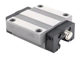
WON H25 series standard bearing block, full ball recirculating bearing, flanged, end seal and inside seal, carbon steel. For use with H25 series rails.
