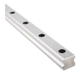
WON H25 series standard rail, carbon steel,  $20 \times 23 \times 400$ mm. For use with H25 series bearings.
