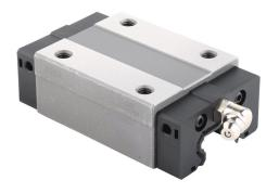
WON H20 series standard bearing block, full ball recirculating bearing, rectangular, end seal, carbon steel. For use with H20 series rails.
