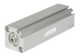
NITRA pneumatic cylinder, compact extruded, 20mm bore, 10mm rod diameter, 100mm stroke, double acting, magnetic piston, tapped end caps mount.
