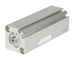
NITRA pneumatic cylinder, compact extruded, 20mm bore, 10mm rod diameter, 75mm stroke, double acting, magnetic piston, tapped end caps mount.
