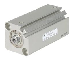
NITRA pneumatic cylinder, compact extruded, 20mm bore, 10mm rod diameter, 50mm stroke, double acting, magnetic piston, tapped end caps mount.
