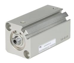
NITRA pneumatic cylinder, compact extruded, 20mm bore, 10mm rod diameter, 40mm stroke, double acting, magnetic piston, tapped end caps mount.
