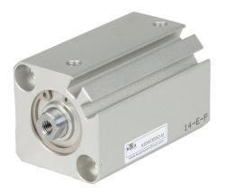
NITRA pneumatic cylinder, compact extruded, 20mm bore, 10mm rod diameter, 30mm stroke, double acting, magnetic piston, tapped end caps mount.
