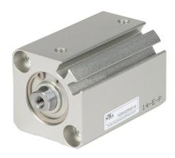
NITRA pneumatic cylinder, compact extruded, 20mm bore, 10mm rod diameter, 25mm stroke, double acting, magnetic piston, tapped end caps mount.
