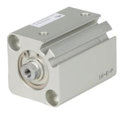
NITRA pneumatic cylinder, compact extruded, 20mm bore, 10mm rod diameter, 20mm stroke, double acting, magnetic piston, tapped end caps mount.
