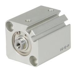
NITRA pneumatic cylinder, compact extruded, 20mm bore, 10mm rod diameter, 15mm stroke, double acting, magnetic piston, tapped end caps mount.
