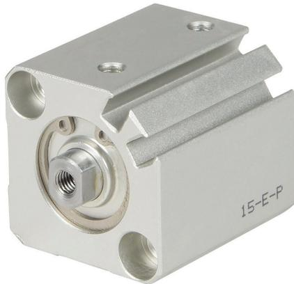
NITRA pneumatic cylinder, compact extruded, 20mm bore, 10mm rod diameter, 10mm stroke, double acting, magnetic piston, tapped end caps mount.
