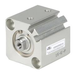
NITRA pneumatic cylinder, compact extruded, 20mm bore, 10mm rod diameter, 5mm stroke, double acting, magnetic piston, tapped end caps mount.
