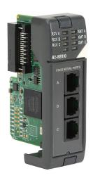
DirectLOGIC DL205 communication module, Do-more protocol, Modbus RTU and ASCII, 3 ports, buffered, (3) RS-232 (RJ12) port(s). For use with Do-more H2 series PLCs or an H2-EBC100-based system connected to a PC.
