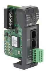
DirectLOGIC DL205 communication module, Do-more protocol, Modbus RTU and ASCII, 3 ports, buffered, (2) RS-232 (RJ12) and (1) RS-422/RS-485 port(s). For use with Do-more H2 series PLCs or an H2-EBC100-based system connected to a PC.
