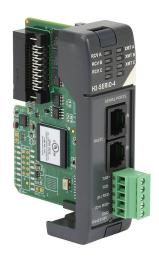
DirectLOGIC DL205 communication module, Do-more protocol, Modbus RTU and ASCII, 3 ports, buffered, (2) RS-232 (RJ12) and (1) RS-422/RS-485 port(s). For use with Do-more H2 series PLCs or an H2-EBC100-based system connected to a PC.
