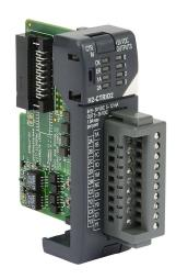
DirectLOGIC DL205 pulse combo module, 250 kHz maximum switching frequency, 8 high-speed input point(s), sinking/sourcing, single-ended encoder input(s), 4 high-speed output point(s), sinking/sourcing, single-ended output(s).
