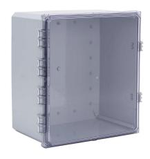
Integra Premium series enclosure, NEMA 1/2/3/3R/3S/4/4X/5/12/13, 18 x 16 x 10in (HxWxD), wall mount, polycarbonate, gray, gloss finish, clear polycarbonate single-door, glass-filled nylon quick-release latch, padlock hasp and staple.
