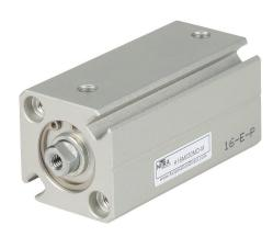
NITRA pneumatic cylinder, compact extruded, 16mm bore, 8mm rod diameter, 30mm stroke, double acting, magnetic piston, tapped end caps mount.
