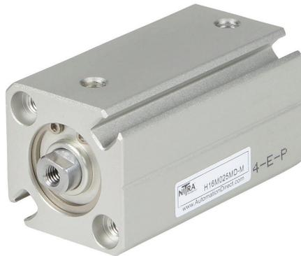
NITRA pneumatic cylinder, compact extruded, 16mm bore, 8mm rod diameter, 25mm stroke, double acting, magnetic piston, tapped end caps mount.
