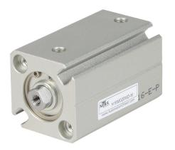
NITRA pneumatic cylinder, compact extruded, 16mm bore, 8mm rod diameter, 20mm stroke, double acting, magnetic piston, tapped end caps mount.
