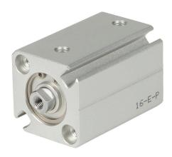
NITRA pneumatic cylinder, compact extruded, 16mm bore, 8mm rod diameter, 15mm stroke, double acting, magnetic piston, tapped end caps mount.
